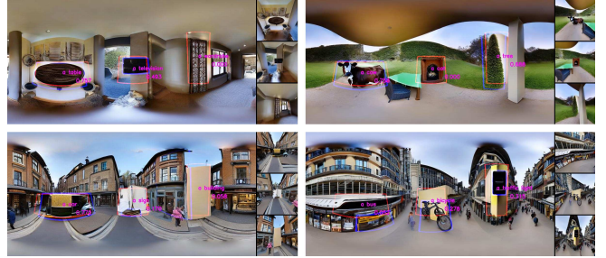
Fig. 5. Various failure-cases of MultiPanFusion, visualizing noise around the objects, unfitting ceilings, wrong objects, and foreground elements merging with the background.
