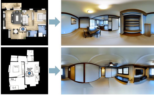
Figure 5. Our Top2Pano model generalizes to both textured floorplans (first row) and hand-drawn sketched floorplans (second row), incorporating stylized [Japanese] control.
