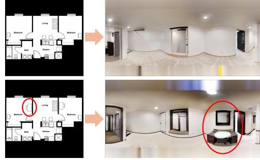
Figure 6. Top2Pano enables panorama manipulation via compositional floorplan editing. In the second row, adding a rectangular object to the floorplan (compared to the first row) leads the model to generate a washstand with a mirror in the panorama.
